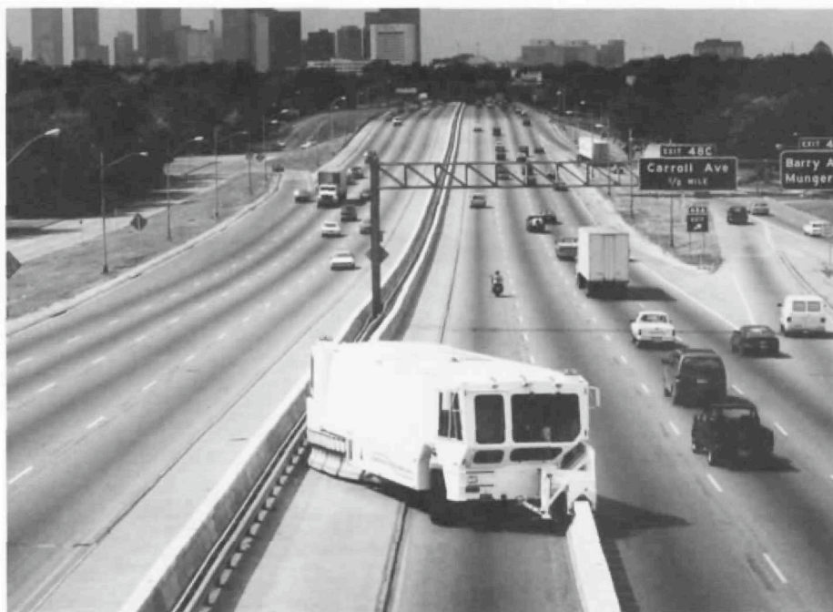
Barrier transfer vehicle, developed by Barrier Systems, Inc., works the R. L. Thornton Freeway in Dallas.
