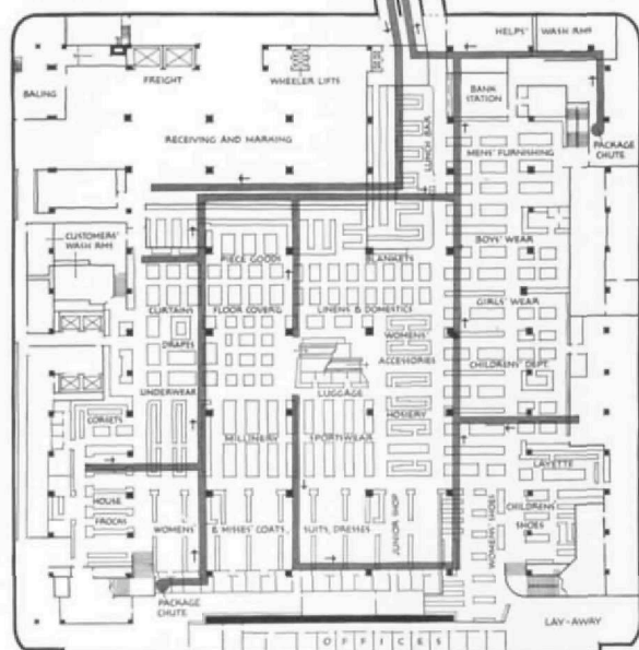
Basement plan showing route of merchandise from truck platform to sorting ring, tunnel under Travis Street, and receiving and marking area in main store. From there it was taken on wheeler lifts to stock receiving areas on each floor.
